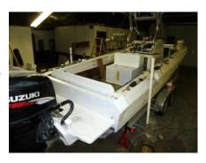
I built a very useful leaning post-live well-ice box-fresh water holding tank-trash bin out of plywood, epoxy and Lexan viewing window, where just a hard leaning post was mounted before. Added jump seats to the back, where wet tail was previously. Now there's room for four guests to sit or someone could lie down at the back end. Plus there's about three extra feet now on back to fish or relax.
