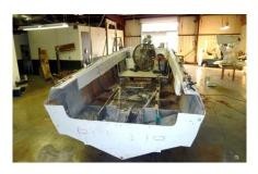
Then I started building new flooring using Baltec Airex panels & epoxy sandwich construction methods. Moved the console forward by 30" to get better balance. Cut out the fish box and applied two layers of insulating foam to its backside. While the floor was out, filled the hollow lifting strakes with crack sealing epoxy, and bolstered all the
